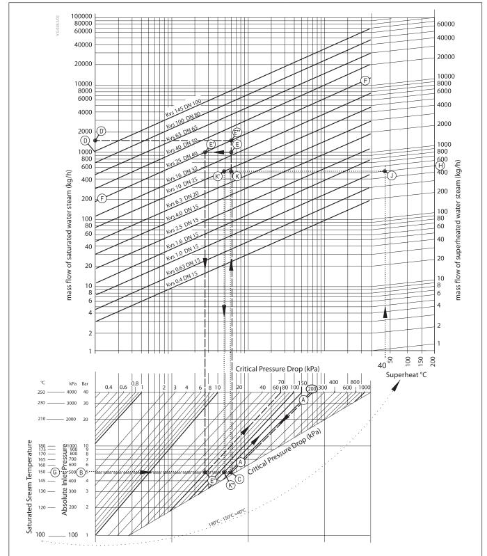
Steam valve sizing is based on 40 % of the absolute steam pressure (immediately upstream of the valve), being dropped across the valve when fully open. At this condition the steam is travelling at or close to its critical velocity (approx. 300 m/s) and throttling will occur over the full valve stroke. If the steam is travelling slower than this then the first part of the valve stroke will merely increase the velocity of the steam without reducing the volumetric flow.
